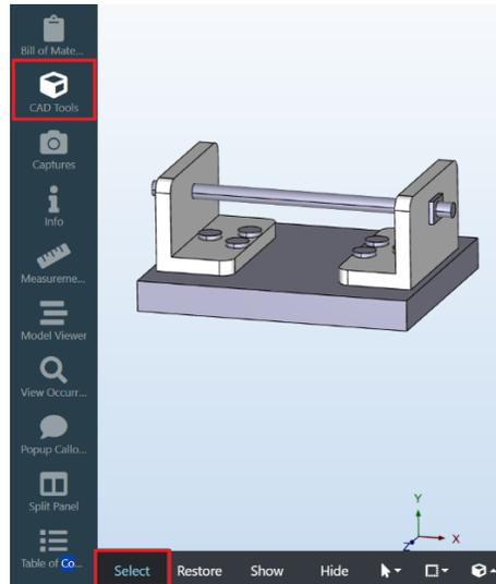
When the Select button is enabled you can perform the multiple selection by single clicking on parts or using the marquee selection tool.
